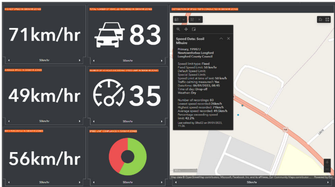
Figure 20 - Screenshot of speed survey dashboard for speed surveys carried out at proposed locations of new crossings on the N4 near Scoil Mhuire, Newtownforbes, Co. Longford.
