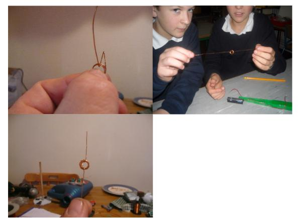
**Note:** Be sure to centre the two tails on either side of the coil. Balance is important.
