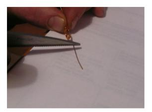
4. Strip 2cm from each end of the lengths of bellwire, shape one end of each piece of bellwire into a loop using the matchstick
